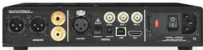
ABOVE: Balanced (XLR) and single-ended (RCA) analogue outs are joined by AES/EBU (XLR), Toslink optical, S/PDIF (coaxial on BNC) and USB digital inputs. The 'Exp' HDMI connection is destined to be enabled by a future firmware update
